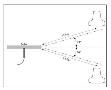
1.1.3 The antenna unit shall be mounted minimum 1 metre from MF-HF, VHF and UHF antennas.
