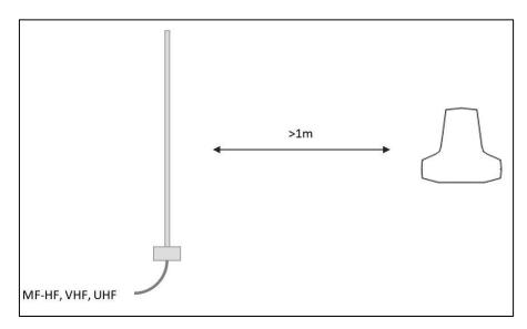
1.1.4 The antenna unit should be installed with a 360° clear view of the sky. However, minor obstructions such as a mast will not degrade the antenna performance severely, if a separation distance larger than 15 times the diameter of the obstruction is kept.
