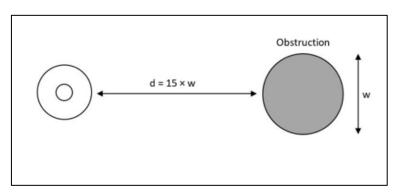
1.1.5 The equipment should be installed and mounted in accordance with the manufacturer's requirements in the technical documentation. If two Iridium antennas are installed, the antennas should be installed such as to ensure electromagnetic compatibility.
